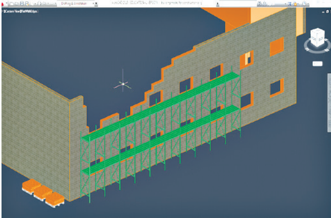
POSSIBLE BIM-M MATERIAL STAGING TOOL.
